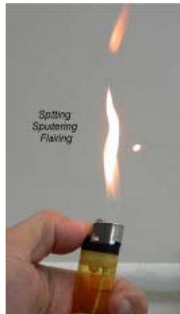
Flame with spitting, sputtering and flaring
